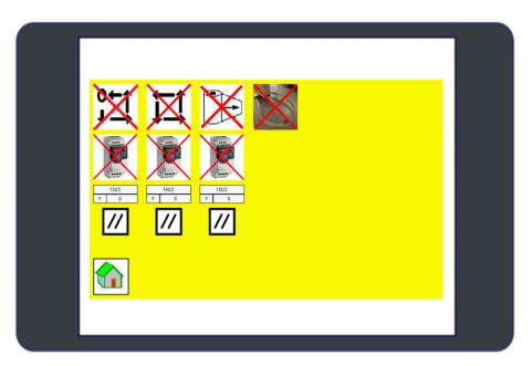
This screen shows malfunctions. They need to be resolved before the machine can be restarted.
